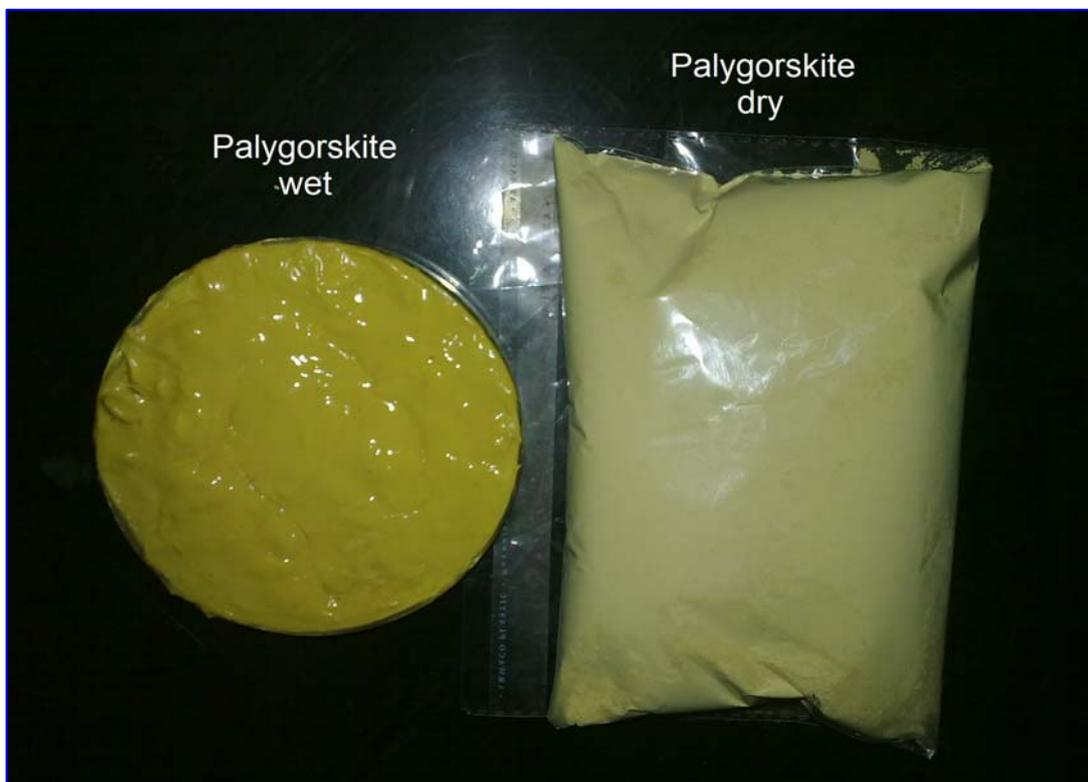
Figure 2-10: Wet (left) and dry samples (right) of separated palygorskite.
