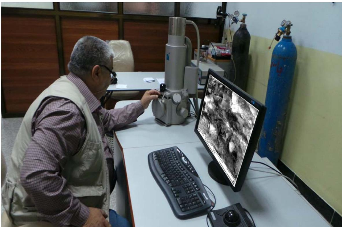
Figure 2-11: Studying the palygorskite mineralogy using SEM at the Nanotechnology and Advance Materials Research Center at the University of Technology with a device type of VIGA TESCAN II SBH MS12.
